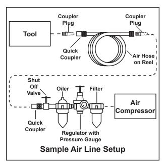
6. Depending on the tool which you will be using with this compressor, you may need to incorporate additional components, such as an in-line oiler, a filter, or a dryer (all sold separately).
